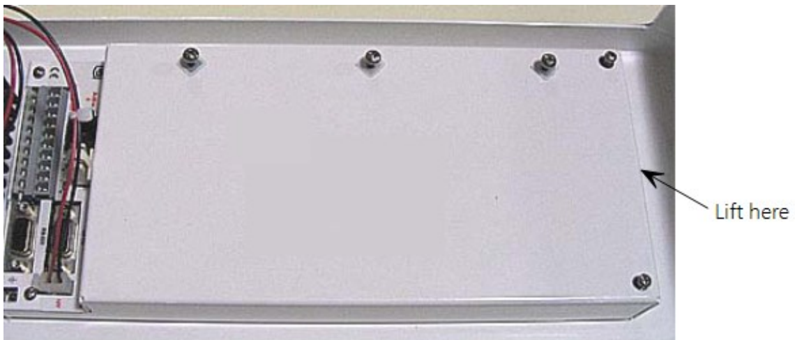
FIGURE 6-14. Removal of the electronics cover
