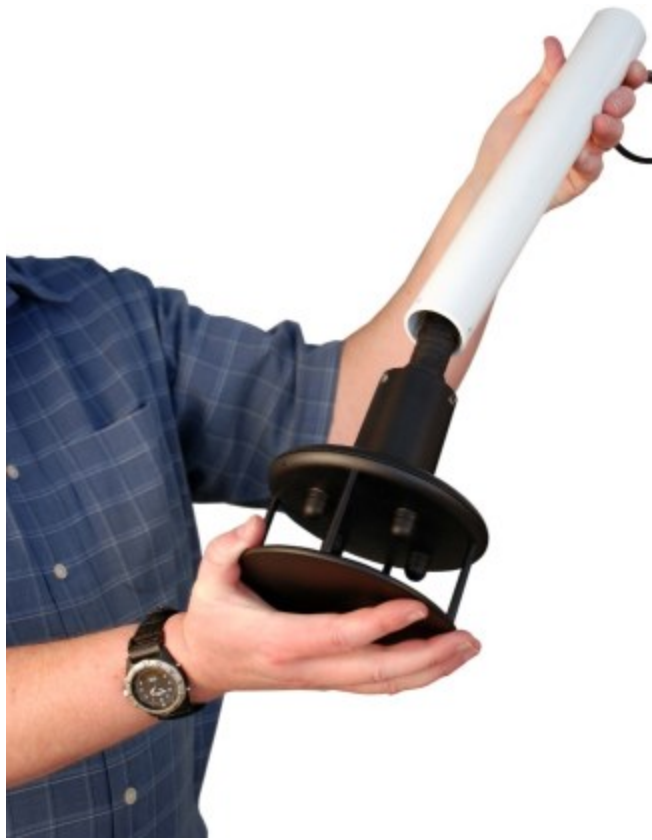
FIGURE 6-17. WindSonic connected to cable
